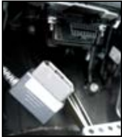
Example of electric running boards being unplugged.
